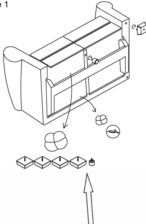
**1. The wood legs and transformer are located at Underneath of the furniture, open the white non-woven bags and get the bolted legs. Please place in hole and tighten with hand clockwise till sungs.**
